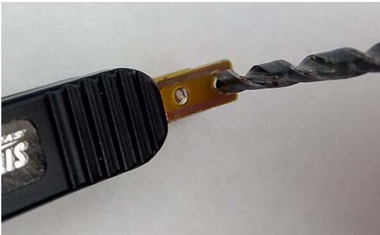
3. Sometimes bits of metal remain stuck in the threads from assembly. These bits can be removed using a tap or one of the screws to clear the threads. Tighten and remove a few times.
