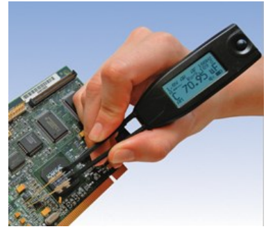
Smart Tweezers LCR-meter simplifies PCB debugging
