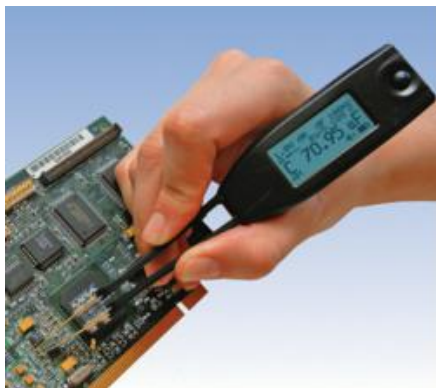
Smart Tweezers LCR-meter simplifies PCB debugging
